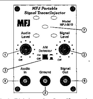
Audio Level: This knob turns the audio amplifier on and controls the speaker volume.
